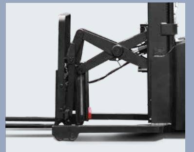
Forks move forward by the scissor structure
