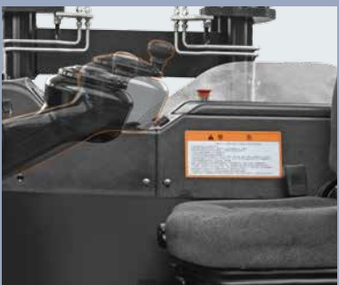
The steering wheel is extensible, so the operator can choose the best driving position
