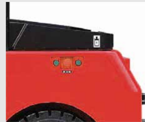
Forward/Reverse inching switch and emergency switch are mounted on the left rear, them make the hook easy and safe
